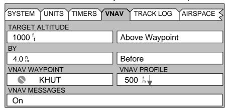
2. Use the Rocker Keypad to highlight the desired field, PRESS ENTER and key in the characters. We have selected 1,000 ft above the KHUT airport 4.0 NM before reaching it. We also would like a 500 ft/min descent rate and have turned the VNAV messages ON.
